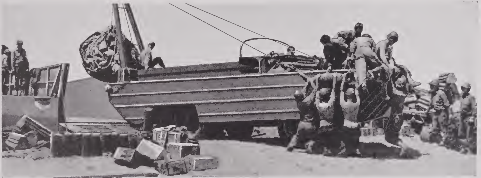
FIGURE 19. Unloading cargo at Sicily by means of DUKW A-frame. Since load is more than 3,000 pounds, counterweight is used on bow of DUKW to prevent its tipping. In case illustrated here, manpower is being used, but it is better to use 1,000 pounds of ammunition or other cargo, or to install brace under pintle hook on DUKW stern.
